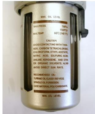
**Figure 2:** Warning label and min/max oil level lines on casing.
